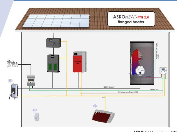
**ASKO**HEAT+ 2.0 screw-in or flanged heater, with **remote control** together with bidirectional meter.
